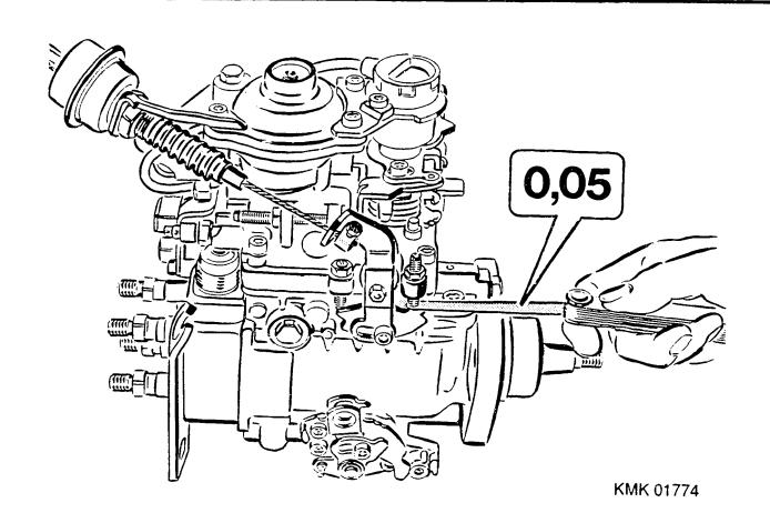
Detach vacuum connection from pneumatic actuator. LFG stop lever must now be positioned against stop for low idle.
